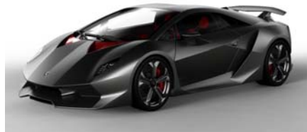
Lamborghini Sesto Elemento with a body made of CFRP, weighs just 999 kg. The vehicle powered by a 562 hp V10 engine and permanent all-wheel drive
